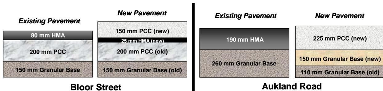
FIGURE 2 Existing and new pavement designs.
