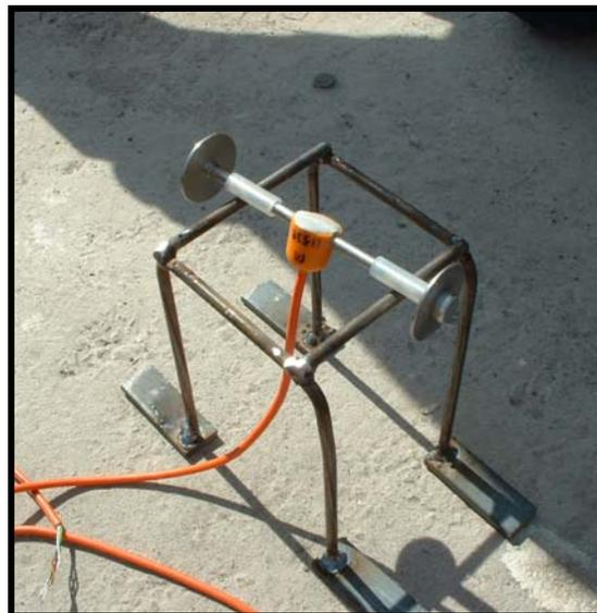
**FIGURE 4 Typical strain gauge installation before paving.**
