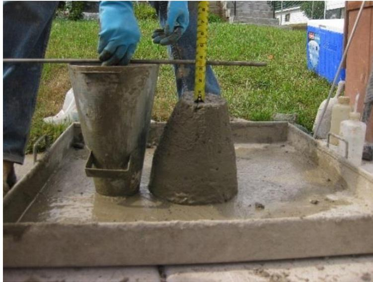
**Figure 4-24 Conducting slump test on Jameston Ave.**
