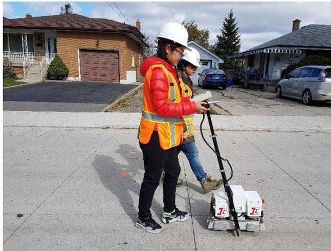
**Figure 5-14 Testing on Jameston Ave. using a SurPRO profiler**
