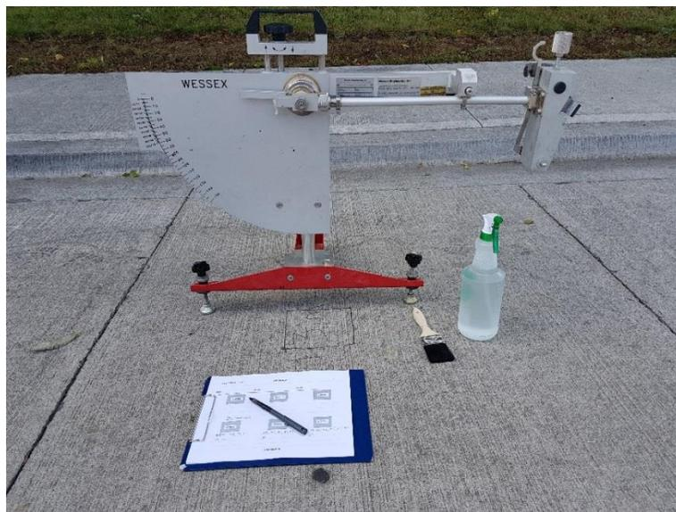
**Figure 5-19 British Pendulum Test Apparatus**
