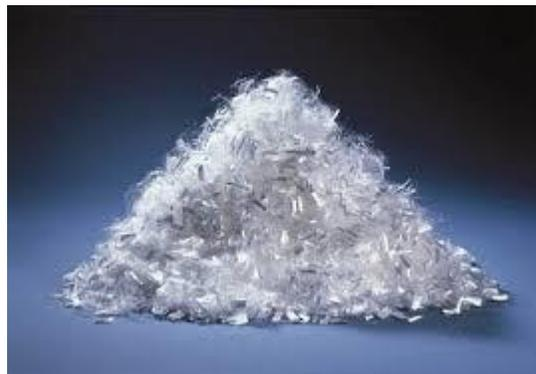
**Figure 2-5 Polypropylene fibres (CEMEX UK Materials Ltd)**
