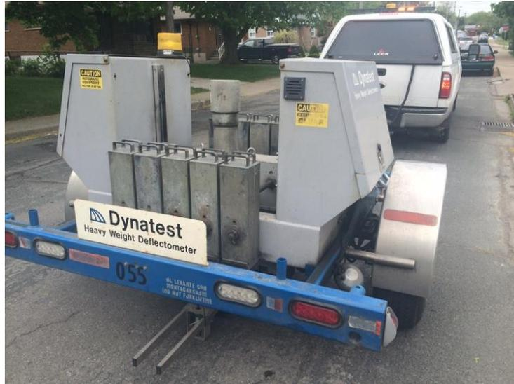
**Figure 3-10 Falling Weight Deflectometer (FWD)**
