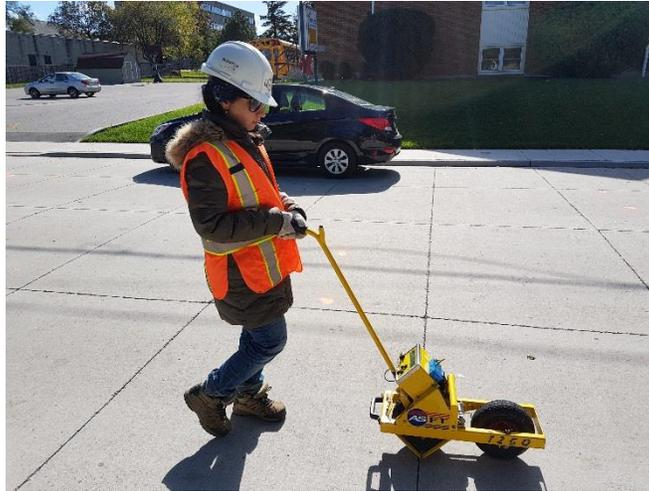
**Figure 5-23 T2GO testing on Jameston Ave. concrete overlay**
