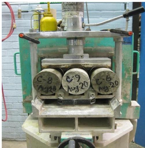
**Figure 4-25 End grinding of concrete cylinders**
