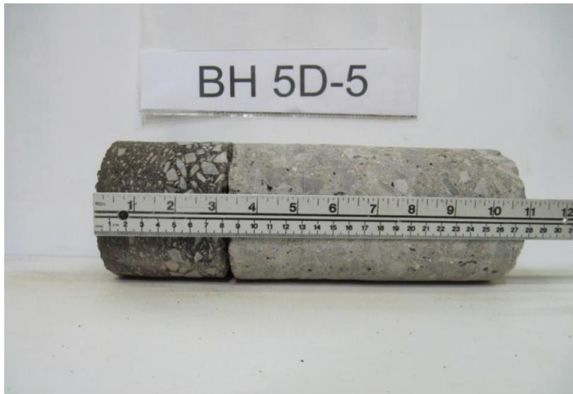
**Figure 3-9 Typical sample core from Jameston Ave.-Section 1
