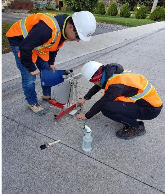
Figure 5-20 British Pendulum testing on Jameston Ave.
