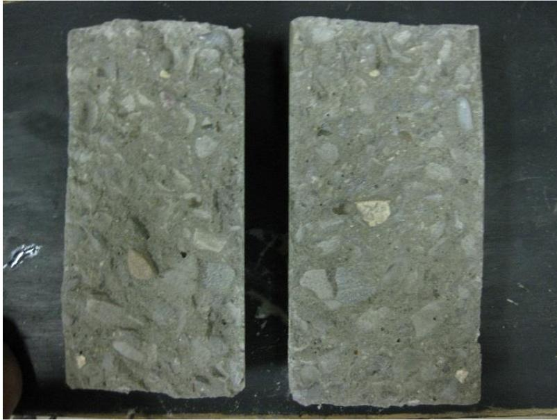
**Figure 4-28 Split cylinder after tensile testing**
