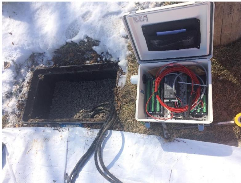
**Figure 4-9 Sub-surface mountbox with instrumentation box and datalogger**
