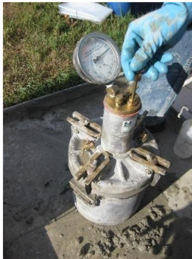
**Figure 4-23 Pressure method testing on Jameston Ave.**
